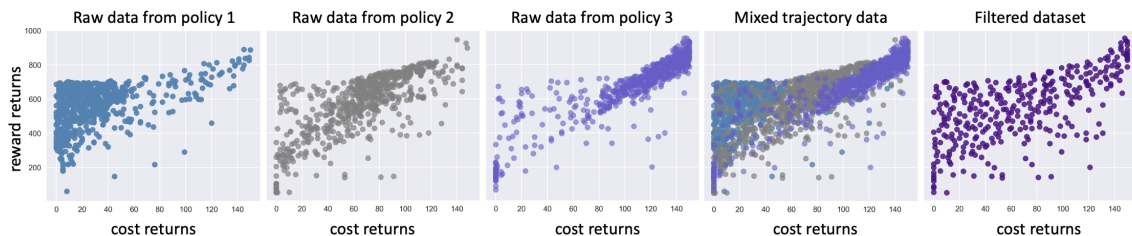
Figure 2: Illustration of the cost-reward plot and data collection from a mixture of experts. Multiple expert policies are trained, the raw data is collected, and a density filter is applied to remove redundant trajectories concentrated within the same region.
